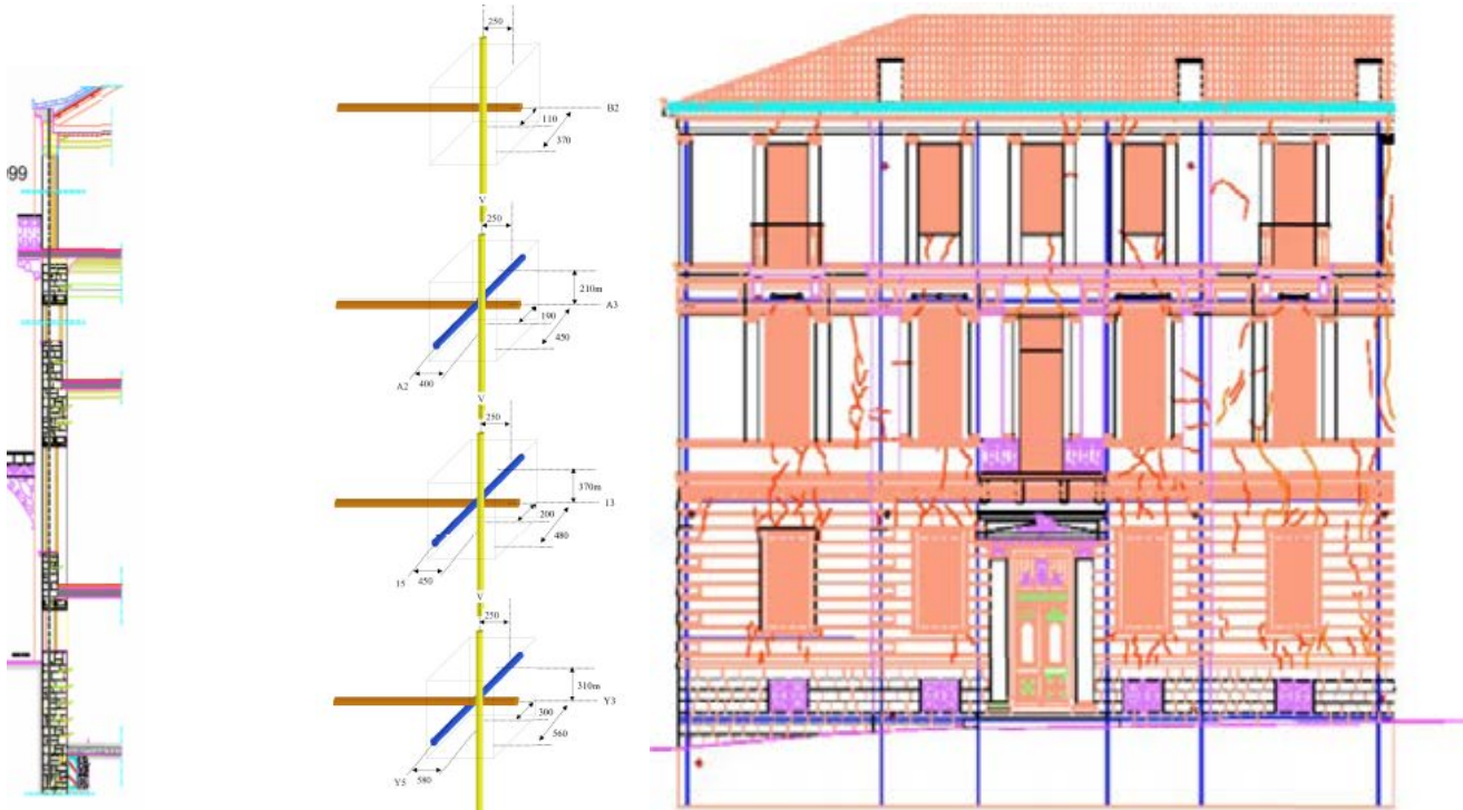
Anchor positions were carefully marked out and drilled with extreme precision to avoid intersecting anchors
