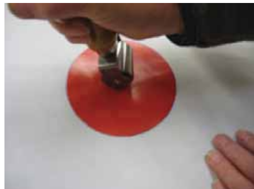
Roll the patch firmly. Allow at least 24 hours before inflation and re-use.
