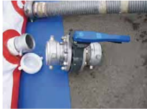
Attach 4" female butterfly valves To each side of dam
