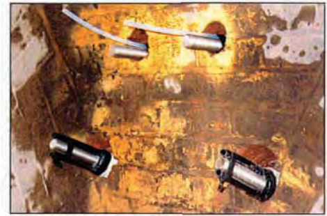
Shear anchors shown at the top and tension anchors at the bottom
