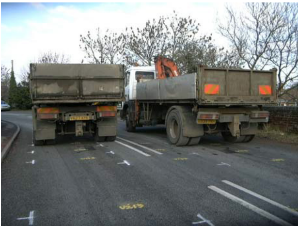
Loading using 11.5 tonnes single axles
